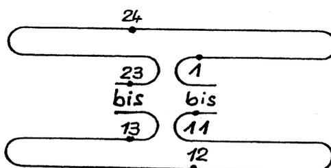
This scheme shows the view on the skirt of the pleated canopy as seen from the container's direction. The points marked with numbers represent the respective suspension lines.
