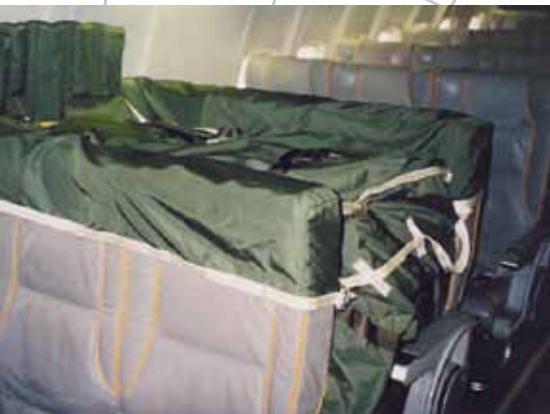
Installed Cargo Container
